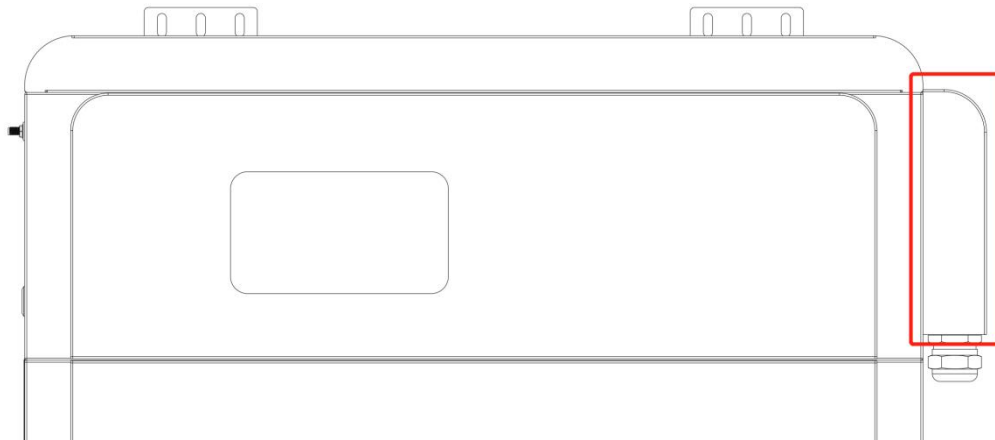
Figure 3.6.1. Removal position of the battery control module
