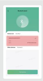
Search for the battery's Bluetooth signal using the serial number on the nameplate.
